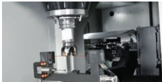
Laser measuring system
